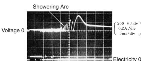
(b) DC Breaking Characteristics of Conventional Power Relays
