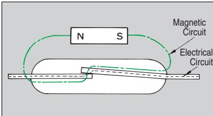
● Magnetic and Electrical Circuits of Bestact
